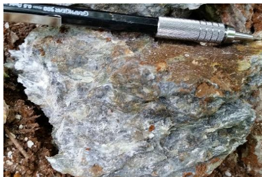
Figure 4. Talc tremolite schist hand sample view.
